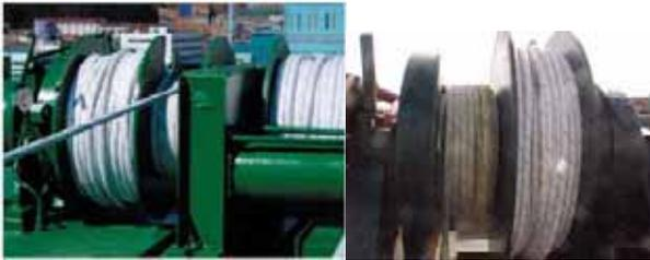
Figure 14. DPX-75 new (left) vs. 6 months in service (right)
