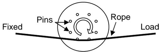
Figure 8. Abrasion Resistance Measurement
