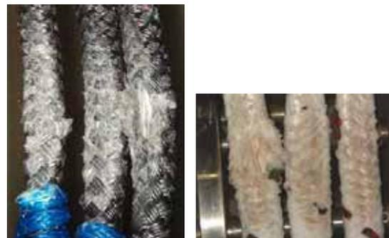
Figure 12. Visual comparison of the Dyneema® fiber jacket (left) and DPX (right) showed similar wear.
