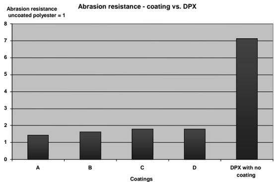
Figure 11. Abrasion resistance improvement through coating on Polyester.
