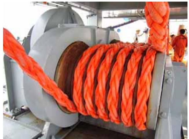
Figure 17. Quantum 8 on a turret pick up winch.
