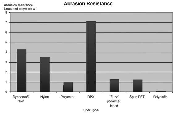
Figure 10. Abrasion resistance of different fiber types.
