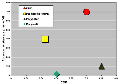
Figure 9. Comparison of Fiber Surface Properties, COF vs. Abrasion resistance
