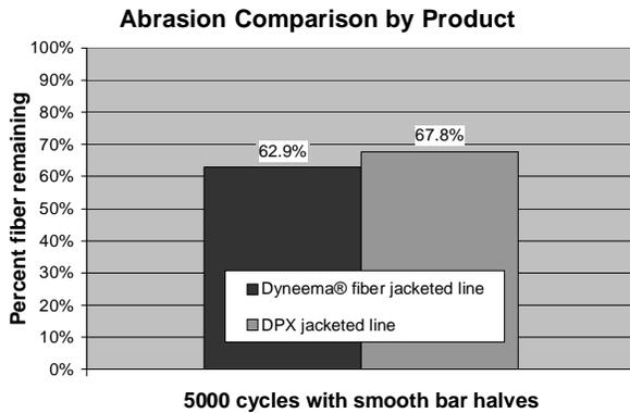
Figure 13. Remaining cover fibers after 5000 abrasion cycles DPX vs. Dyneema® fiber, showing comparable abrasion resistance
