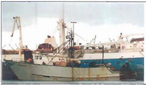
Figure 13 Port view of TENACITY (1996) Note addition of processing space on main deck.
