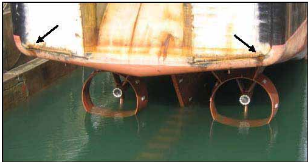
Figure 17: Photograph of the stern taken in 2005 showing water draining from outer transom
