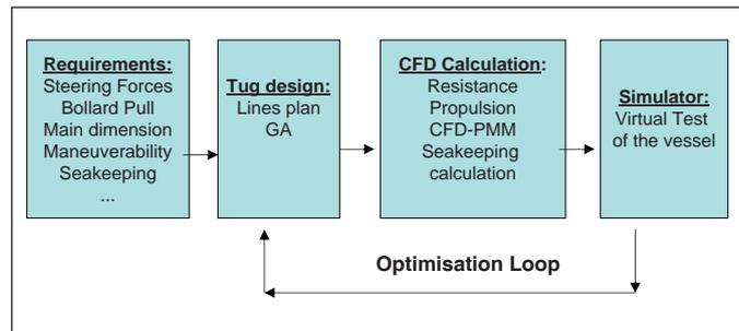
Figure 7: Design loop, based on CFD and simulator.
