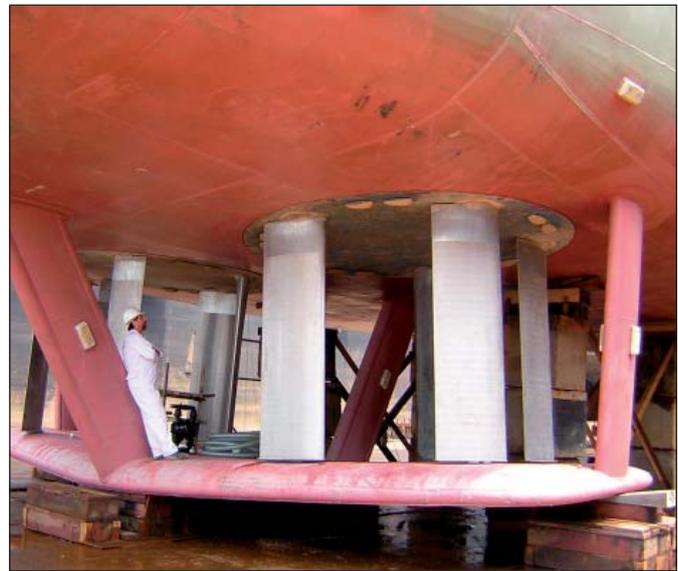
Figure 6: Installation of two VSPs in a VWT.
