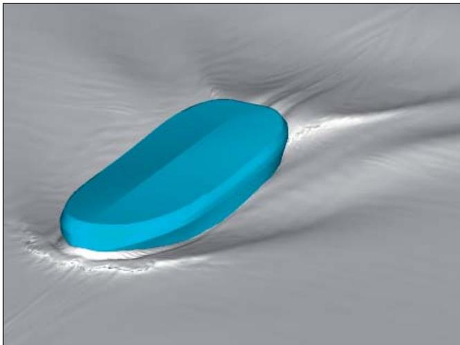
Figure 9: Calculated free surface of manoeuvring VWT.
