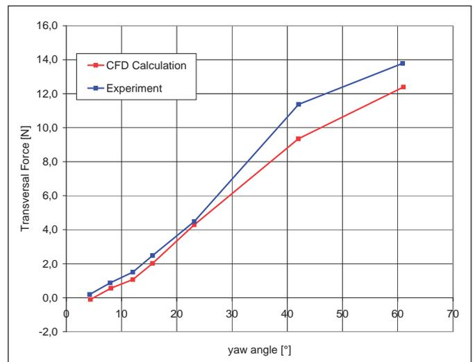
Figure 11: Transversal force as a function of the yaw angle, comparison of measurement and calculation, sailing VSP ahead;  $U = 2$  knots.
