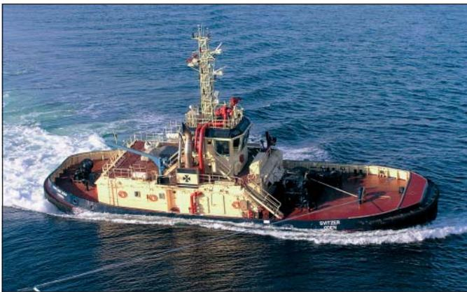
Figure 4: VWT Oden (Svitzer) in escort mode.
