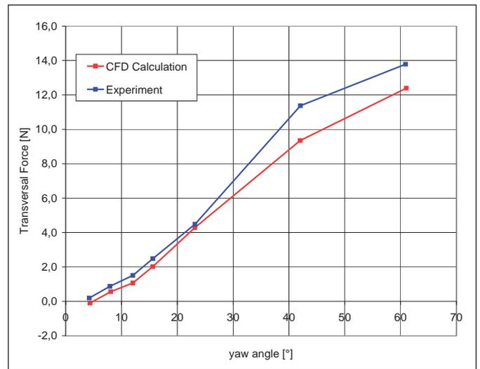
Figure 10: Resistance as a function of the yaw angle, comparison of measurement and calculation, sailing VSP ahead;  $U = 2$  knots.
