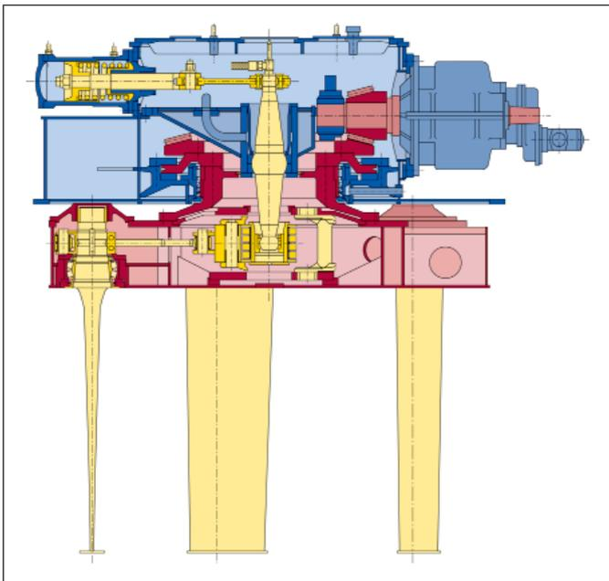
Figure 5: Sectional drawing of a Voith Schneider Propeller.
